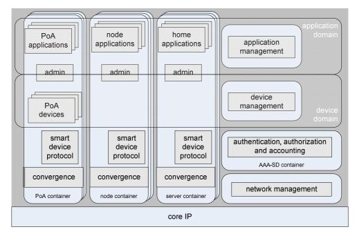
Figure 9.2: TR-50 High Level System Architecture
