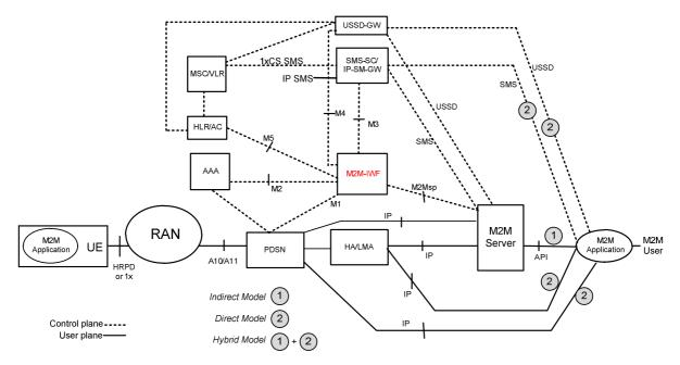
Figure 12.6: 3GPP2 Enhanced Network Architecture to Support M2M
