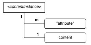
Figure 8.13: Structure of <contentInstance> resource
