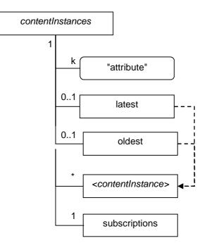
Figure 8.12: Structure of contentInstances resource
