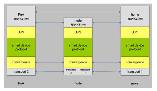
Figure 9.1: TR-50 Conceptual Protocol Stack
