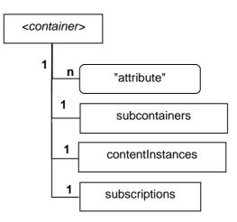
Figure 8.11: Structure of <container> resource
