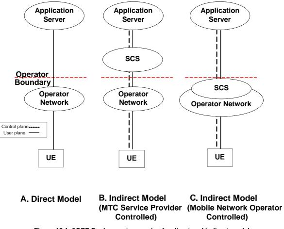
Figure 12.1: 3GPP Deployment scenarios for direct and indirect model
