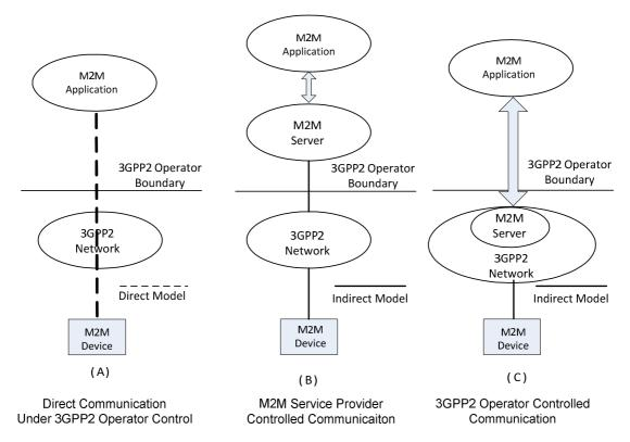
Figure 12.4: M2M Application to M2M Device Communication Models
