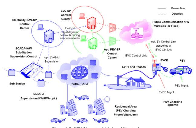
Figure 9.5: PEV Charging High Level Illustration
