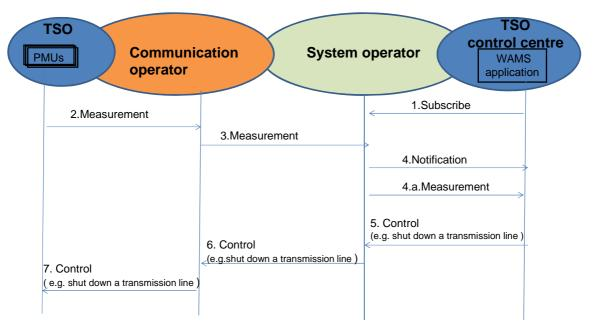
Figure 5.1: An example flow for the TSO scenario
