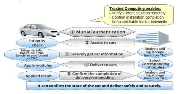
Figure 10.3: Remote Maintenance Flow
