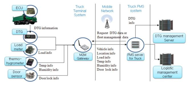
Figure 10.7: Normal Flow - Fleet Management Service (Truck)
