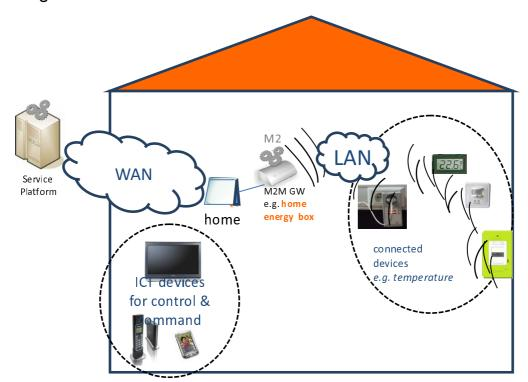
Figure 9.2: Home Energy Management System High Level Illustration
