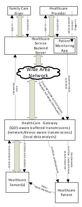
Figure 7.6: Healthcare Gateway High Level Illustration
