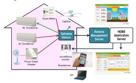
Figure 9.3: Home Energy Management System High Level Illustration
