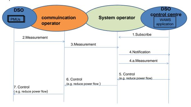
Figure 5.2: An example flow for DSO scenario
