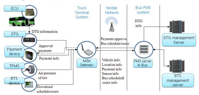
Figure 10.8: Normal Flow - Fleet Management Service (Bus)
