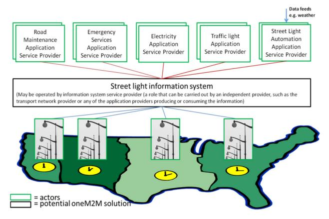
Figure 8.1: Street Light Automation High Level Illustration
