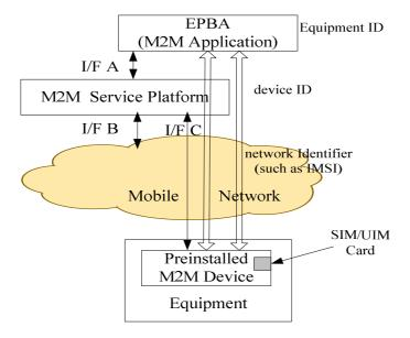
Figure 11.19: High Level Illustration
