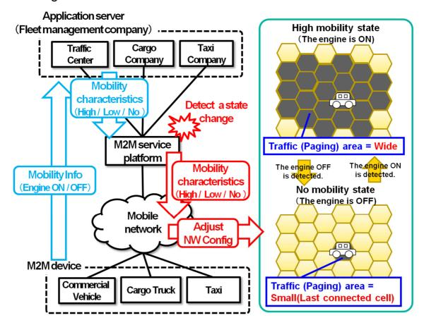
Figure 11.8: High Level Illustration - Optimizing mobility management parameters
