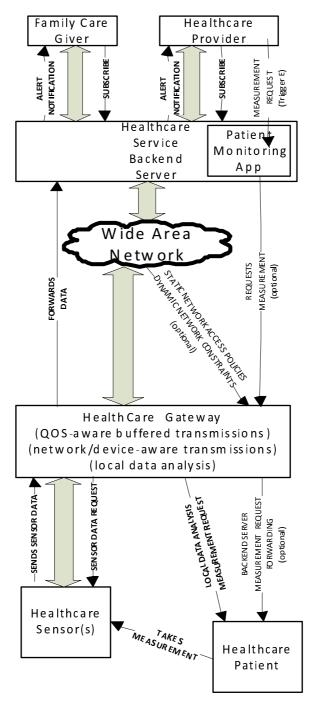
Figure 7.4: Local Gateway Data Analysis Flow
