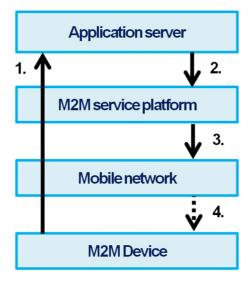
Figure 11.7: Normal Flow - Optimizing mobility management parameters
