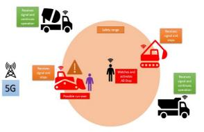
"All-Stop" in Mining and Construction Site Applications -Source: ISO TC 127 SC2 WG 22 – Autonomous Machine Safety
